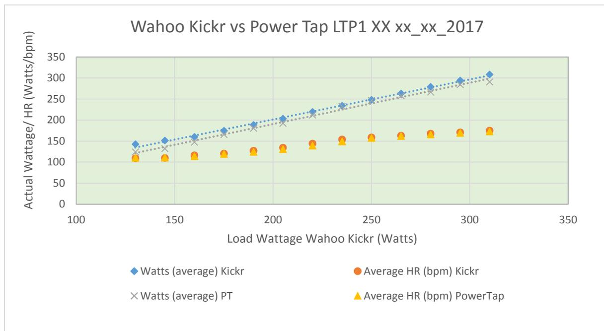
From the comparison of nominal calibrated Wahoo KICKR power measurements against your Power Tap mobile ergometer we can see there is a small although constant linear discrepancy throughout the power range assessed, average difference of -10W (-5.2% average RE). This difference seems to be more significant at the lower and upper end of the power range (<200W, >300W). For that reason you should correct your scaled lactate threshold training zones as necessary for use with that power meter only.
